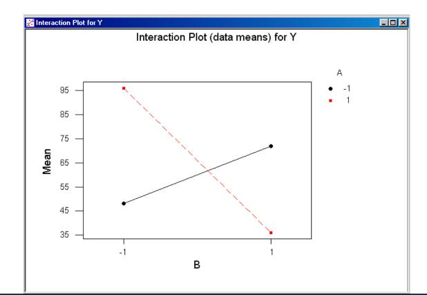
Parallel lines indicate no interaction; the less parallel, the higher the degree of interaction
