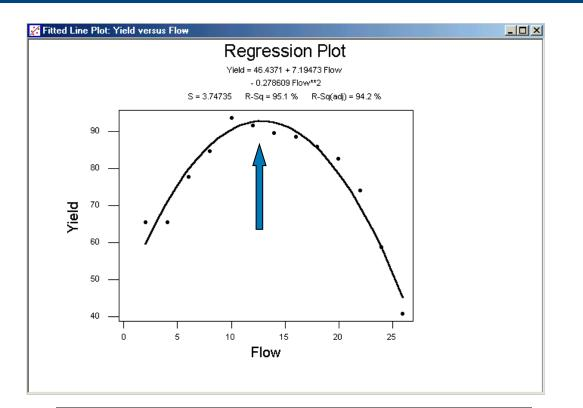
Regression analysis provides equation which can be solved for flow
