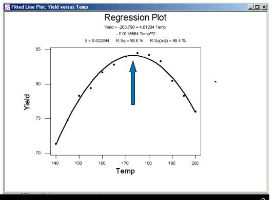
Regression analysis provides an equation which can be solved for temperature
