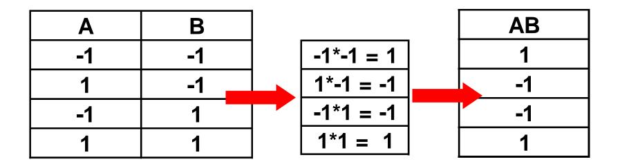
Finding the interaction levels in a coded design is as simple as multiplying one times one
